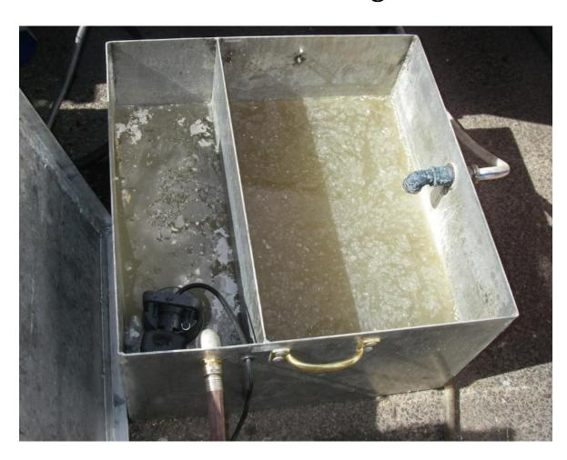
Solution: This tote will work a lot better than a grease trap for the vendors that have a pump inside of their trailers. This tote is pumped out whenever it fills with grey water.
