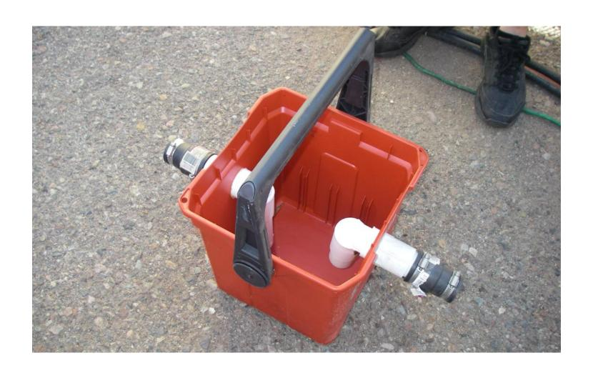
Not a preferred grease trap. The outlet baffle wall can be easily removed by lifting straight up, this will allow accumulated grease to flow with water to the sewer, defeating the purpose. Trap needs two walls.
